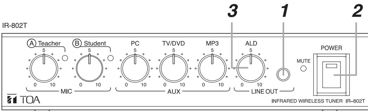
**Step 1.** Connect the Assistive listening system to the ALD output terminal on the front panel.
