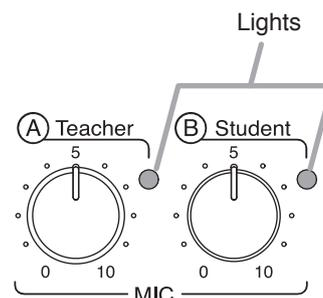
**Step 3.** Adjust the volume control knob for an appropriate output sound.
