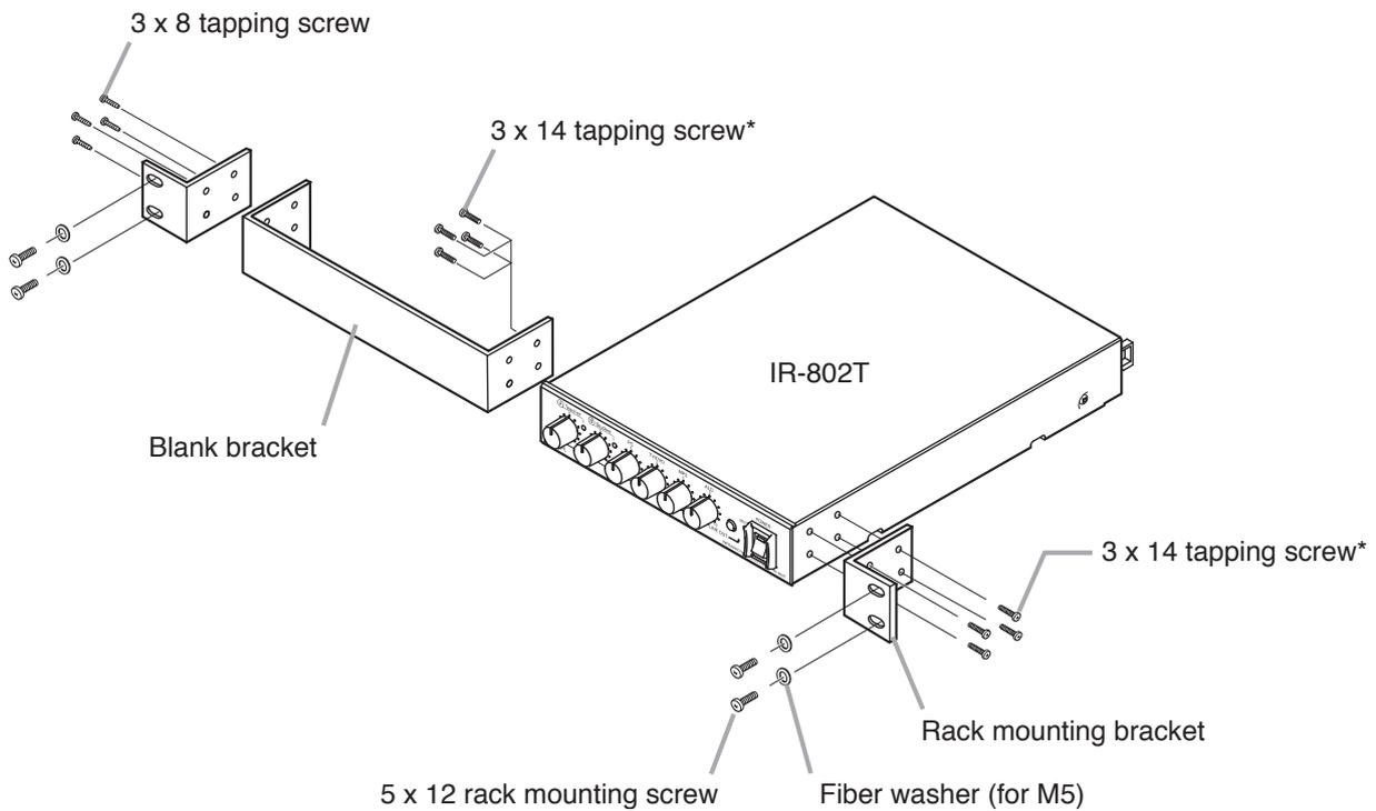
\* Secure the brackets with the screws supplied with the MB-15B-BK after removing the case holding screws, which are no longer used.
